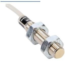
ProSense inductive proximity sensor, tubular, 8mm diameter x 40.4mm body, nickel-plated brass housing, PNP, N.O. output, 1.5mm sensing distance, flush, 1000 Hz switching frequency, IP67, pigtail.
