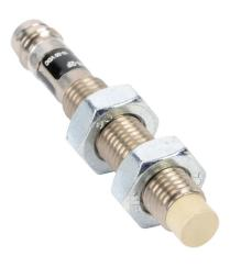
ProSense inductive proximity sensor, tubular, 8mm diameter x 53.9mm body, nickel-plated brass housing, NPN, N.O. output, 2mm sensing distance, non-flush, 1000 Hz switching frequency, IP67, 3-pin M8 quick-disconnect.
