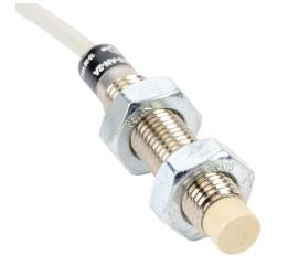
ProSense inductive proximity sensor, tubular, 8mm diameter x 44.4mm body, nickel-plated brass housing, NPN, N.O. output, 2mm sensing distance, non-flush, 1000 Hz switching frequency, IP67, pigtail.
