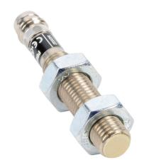
ProSense inductive proximity sensor, tubular, 8mm diameter x 49.9mm body, nickel-plated brass housing, NPN, N.O. output, 1.5mm sensing distance, flush, 1000 Hz switching frequency, IP67, 3-pin M8 quick-disconnect.
