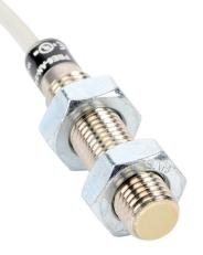
ProSense inductive proximity sensor, tubular, 8mm diameter x 40.4mm body, nickel-plated brass housing, NPN, N.O. output, 1.5mm sensing distance, flush, 1000 Hz switching frequency, IP67, pigtail.
