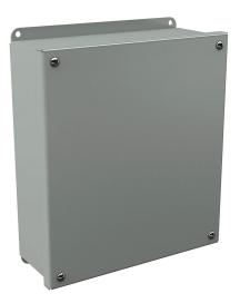
Wiegmann pushbutton enclosure, blank cover, NEMA 4/12/13, 10 x 9 x 3in (HxWxD), wall mount, carbon steel, ANSI 61 gray, powder coat finish, screw cover.
