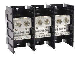
Edison open terminal block, 760A, 3-pole, line side: 2 openings accept 500 MCM to 6 AWG, load side: 12 openings accept 4AWG to 14 AWG, panel mount, UL 1059 recognized.
