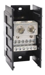
Edison open terminal block, 760A, 1-pole, line side: 2 openings accept 500 MCM to 6 AWG, load side: 12 openings accept 4AWG to 14 AWG, panel mount, UL 1059 recognized.
