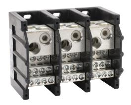
Edison open terminal block, 570A, 3-pole, line side: 2 openings accept 300 MCM to 4 AWG, load side: 12 openings accept 4AWG to 14 AWG, panel mount, UL 1059 recognized.
