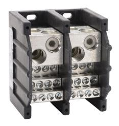
Edison open terminal block, 570A, 2-pole, line side: 2 openings accept 300 MCM to 4 AWG, load side: 12 openings accept 4AWG to 14 AWG, panel mount, UL 1059 recognized.
