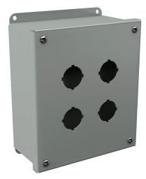
Wiegmann pushbutton enclosure, 4 holes, 30mm, NEMA 4/12/13, 7 x 6 x 3in (HxWxD), wall mount, carbon steel, ANSI 61 gray, powder coat finish, screw cover.
