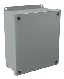
Wiegmann pushbutton enclosure, blank cover, NEMA 4/12/13, 7 x 6 x 3in (HxWxD), wall mount, carbon steel, ANSI 61 gray, powder coat finish, screw cover.
