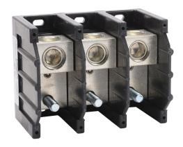
Edison open terminal block, 380A, 3-pole, line side: 1 opening accepts 500 MCM to 6 AWG, load side: 3/8-16 X 1 stud, panel mount, UL 1059 recognized.
