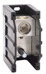
Edison open terminal block, 380A, 1-pole, line side: 1 opening accepts 500 MCM to 6 AWG, load side: 3/8-16 X 1 stud, panel mount, UL 1059 recognized.
