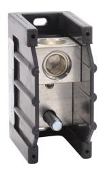
Edison open terminal block, 380A, 1-pole, line side: 1 opening accepts 500 MCM to 6 AWG, load side: 3/8-16 X 1 stud, panel mount, UL 1059 recognized.
