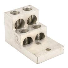
Penn-Union mechanical lug, panelboard, tin-plated aluminum, 600V, 4 openings, (1) 1/0 AWG-750 MCM stranded copper or aluminum, AL9CU.
