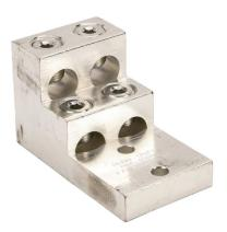
Penn-Union mechanical lug, panelboard, tin-plated aluminum, 600V, 4 openings, (1) 2 AWG-600 MCM stranded copper or aluminum, AL9CU.
