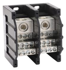
Edison open terminal block, 310A, 2-pole, line side: 1 opening accepts 350 MCM to 4 AWG, load side: 12 openings accept 4AWG to 12 AWG, panel mount, UL 1059 recognized.
