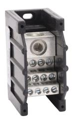
Edison open terminal block, 310A, 1-pole, line side: 1 opening accepts 350 MCM to 4 AWG, load side: 12 openings accept 4AWG to 12 AWG, panel mount, UL 1059 recognized.
