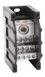
Edison open terminal block, 310A, 1-pole, line side: 1 opening accepts 350 MCM to 4 AWG, load side: 12 openings accept 4AWG to 12 AWG, panel mount, UL 1059 recognized.
