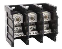
Edison open terminal block, 310A, 3-pole, line side: 1 opening accepts 350 MCM to 4 AWG, load side: 6 openings accept 4 AWG to 12 AWG, panel mount, UL 1059 recognized.
