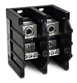
Edison open terminal block, 310A, 2-pole, line side: 1 opening accepts 350 MCM to 4 AWG, load side: 6 openings accept 4 AWG to 12 AWG, panel mount, UL 1059 recognized.
