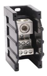
Edison open terminal block, 310A, 1-pole, line side: 1 opening accepts 350 MCM to 4 AWG, load side: 6 openings accept 4 AWG to 12 AWG, panel mount, UL 1059 recognized.
