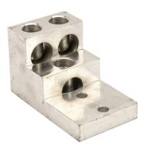
Penn-Union mechanical lug, panelboard, tin-plated aluminum, 600V, 3 openings, (1) 1/0 AWG-750 MCM stranded copper or aluminum, AL9CU.
