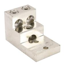
Penn-Union mechanical lug, panelboard, tin-plated aluminum, 600V, 3 openings, (1) 2 AWG-600 MCM stranded copper or aluminum, AL9CU.
