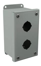
Wiegmann pushbutton enclosure, 2 holes, 30mm, NEMA 4/12/13, 6 x 3 x 3in (HxWxD), wall mount, carbon steel, ANSI 61 gray, powder coat finish, screw cover.
