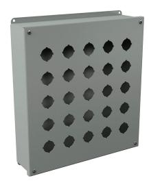
Wiegmann pushbutton enclosure, 25 holes, 30mm, NEMA 12, 14 x 13 x 3in (HxWxD), wall mount, carbon steel, ANSI 61 gray, powder coat finish, screw cover.
