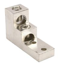
Penn-Union mechanical lug, panelboard, tin-plated aluminum, 600V, 2 openings, (1) 1/0 AWG-750 MCM stranded copper or aluminum, AL9CU.
