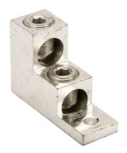
Penn-Union mechanical lug, panelboard, tin-plated aluminum, 600V, 2 openings, (1) 6 AWG-350 MCM stranded copper or aluminum, AL9CU.
