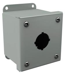
Wiegmann pushbutton enclosure, 1 hole, 30mm, NEMA 4/12/13, 4 x 3 x 3in (HxWxD), wall mount, carbon steel, ANSI 61 gray, powder coat finish, screw cover.
