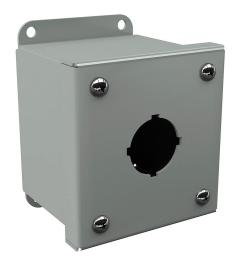
Wiegmann pushbutton enclosure, 1 hole, 30mm, NEMA 4/12/13,  $4 \times 3 \times 3$  in (HxWxD), wall mount, carbon steel, ANSI 61 gray, powder coat finish, screw cover.
