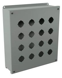
Wiegmann pushbutton enclosure, 16 holes, 30mm, NEMA 12, 12 x 11 x 3in (HxWxD), wall mount, carbon steel, ANSI 61 gray, powder coat finish, screw cover.
