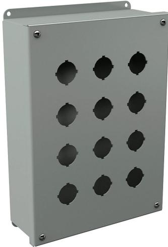
Wiegmann pushbutton enclosure, 12 holes, 30mm, NEMA 4/12/13, 12 x 9 x 3in (HxWxD), wall mount, carbon steel, ANSI 61 gray, powder coat finish, screw cover.
