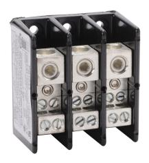
Edison open terminal block, 175A, 3-pole, line side: 1 opening accepts 2/0 AWG to 8 AWG, load side: 4 openings accept 4AWG to 14 AWG, panel mount, UL 1059 recognized.
