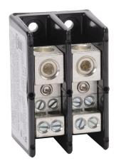
Edison open terminal block, 175A, 2-pole, line side: 1 opening accepts 2/0 AWG to 8 AWG, load side: 4 openings accept 4AWG to 14 AWG, panel mount, UL 1059 recognized.
