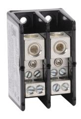
Edison open terminal block, 175A, 2-pole, line side: 1 opening accepts 2/0 AWG to 8 AWG, load side: 4 openings accept 4AWG to 14 AWG, panel mount, UL 1059 recognized.
