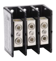
Edison open terminal block, 175A, 3-pole, line side: 1 opening accepts 2/0 AWG to 8 AWG, load side: 1 opening accepts 2/0 AWG to 8 AWG, panel mount, UL 1059 recognized.
