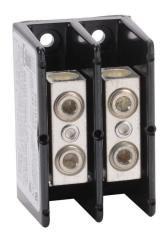
Edison open terminal block, 175A, 2-pole, line side: 1 opening accepts 2/0 AWG to 8 AWG, load side: 1 opening accepts 2/0 AWG to 8 AWG, panel mount, UL 1059 recognized.
