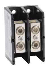
Edison open terminal block, 175A, 2-pole, line side: 1 opening accepts 2/0 AWG to 8 AWG, load side: 1 opening accepts 2/0 AWG to 8 AWG, panel mount, UL 1059 recognized.
