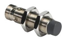
AchieVe inductive proximity sensor, tubular, 12mm diameter x 45mm body, nickel-plated brass housing, PNP, N.O. output, 4mm sensing distance, non-flush, 2 kHz switching frequency, IP67, 4-pin M12 quick-disconnect.
