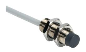
AchieVe inductive proximity sensor, tubular, 12mm diameter x 35mm body, nickel-plated brass housing, PNP, N.O. output, 4mm sensing distance, non-flush, 2 kHz switching frequency, IP67, pigtail.
