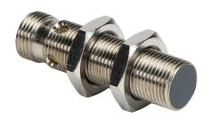
AchieVe inductive proximity sensor, tubular, 12mm diameter x 45mm body, nickel-plated brass housing, PNP, N.O. output, 2mm sensing distance, flush, 3 kHz switching frequency, IP67, 4-pin M12 quick-disconnect.
