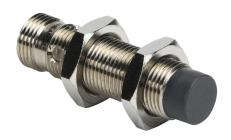
AchieVe inductive proximity sensor, tubular, 12mm diameter x 45mm body, nickel-plated brass housing, NPN, N.O. output, 4mm sensing distance, non-flush, 2 kHz switching frequency, IP67, 4-pin M12 quick-disconnect.
