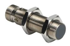
AchieVe inductive proximity sensor, tubular, 12mm diameter x 45mm body, nickel-plated brass housing, NPN, N.O. output, 2mm sensing distance, flush, 3 kHz switching frequency, IP67, 4-pin M12 quick-disconnect.
