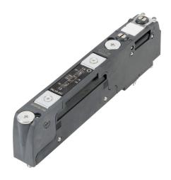
NITRA solenoid valve, 5-way, 3-position, center closed, double solenoid, reinforced technopolymer body, IP65, locking manual override, Cv=0.49, 12-24 VDC.
