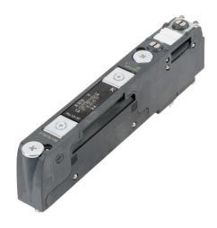
NITRA solenoid valve, 5-way, 2-position, double solenoid, reinforced technopolymer body, IP65, locking manual override, Cv=0.7, 12-24 VDC.
