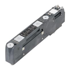
NITRA solenoid valve, modular, 3-way, 2-position, (2) N.C., single solenoid spring return, reinforced technopolymer body, IP65, locking manual override, Cv=0.64, 12-24 VDC.
