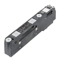
NITRA solenoid valve, modular, 3-way, 2-position, (1) N.C. / (1) N.O., single solenoid spring return, reinforced technopolymer body, IP65, locking manual override, Cv=0.64, 12-24 VDC.
