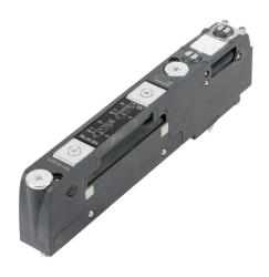
NITRA solenoid valve, modular, 3-way, 2-position, (2) N.O., single solenoid spring return, reinforced technopolymer body, IP65, locking manual override, Cv=0.64, 12-24 VDC.
