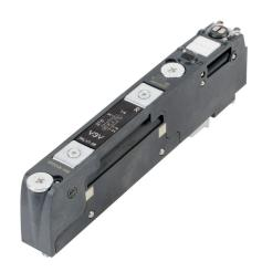
NITRA solenoid bank shut-off pressure relief valve, 5-way, 2-position, single solenoid spring return, reinforced technopolymer body, IP65, locking manual override, Cv=1.07, 12-24 VDC.
