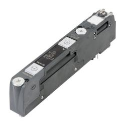
NITRA solenoid valve, 5-way, 2-position, single solenoid spring return, reinforced technopolymer body, IP65, locking manual override, Cv=0.7, 12-24 VDC.
