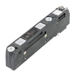
NITRA solenoid valve, modular, 3-way, 2-position, (1) high-flow N.C., single solenoid spring return, reinforced technopolymer body, IP65, locking manual override, Cv=1.28, 12-24 VDC.
