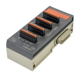
NITRA discrete input module, 16-point, 12-24 VDC, PNP/NPN, 1 common(s), 16 point(s) per common, IP40. For use with PAL series. Mounting hardware included. Requires PAL-EIP bus coupler.
