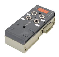
NITRA analog output module, 4-channel, current/voltage, 15-bit, output current signal range(s) of 0-20 mA and 4-20 mA, output voltage signal range(s) of 0-5 VDC, +/- 5 VDC, 0-10 VDC and +/-10 VDC, IP65.
