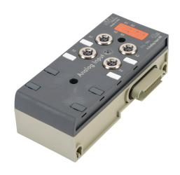
NITRA analog input module, 4-channel, current/voltage, 15-bit, input current signal range(s) of 0-20 mA, 4-20 mA, input voltage signal range(s) of 0-5 VDC, 0-10 VDC, +/- 5 VDC, +/- 10 VDC, IP65.
